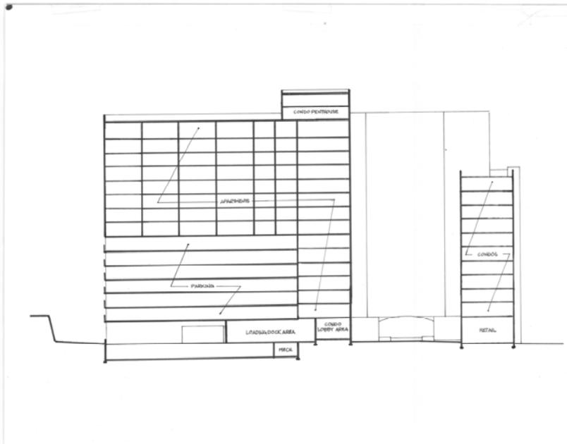
Figure 4: Building section showing occupancies per floor.
